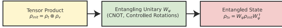
Figure 4: Cross-modal entanglement. Independent text and image states are fused by an entangling unitary W_\psi (e.g., CNOT or controlled rotations) to produce the joint state \rho_{tv} , enabling quantum-native dependency modeling in Hilbert space.
