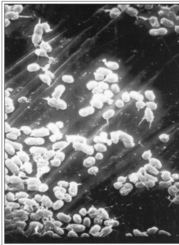
**Figure 1.** Scanning electron microscopy (Magnification = 5000x) demonstrating *P. aeruginosa* bacterial biofilm on a biomaterial surface (polyurethane).
