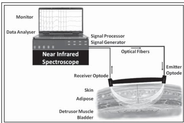
**Figure 2.** The configuration of a NIRS system for transcutaneous interrogation of the bladder detrusor; illustrating the 'banana' shape of the photon path through tissue between the emitter and receiver of the optode, and the effective depth of penetration for NIRS - approximately half the distance chosen to separate the emitter and receiver on the skin surface.
