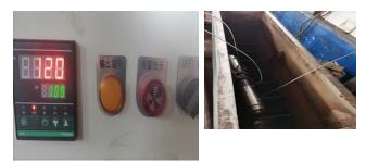
Fig.10 High temperature insulation test equipment
