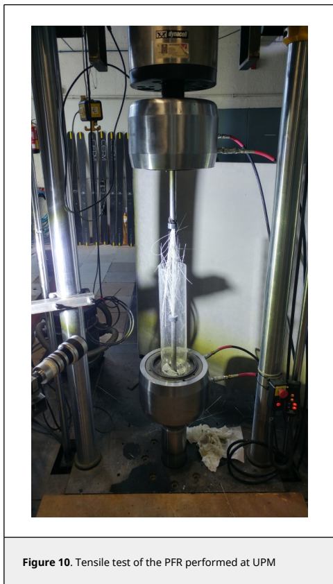
Figure 10 shows a typical bar tested at UPM after failure.
