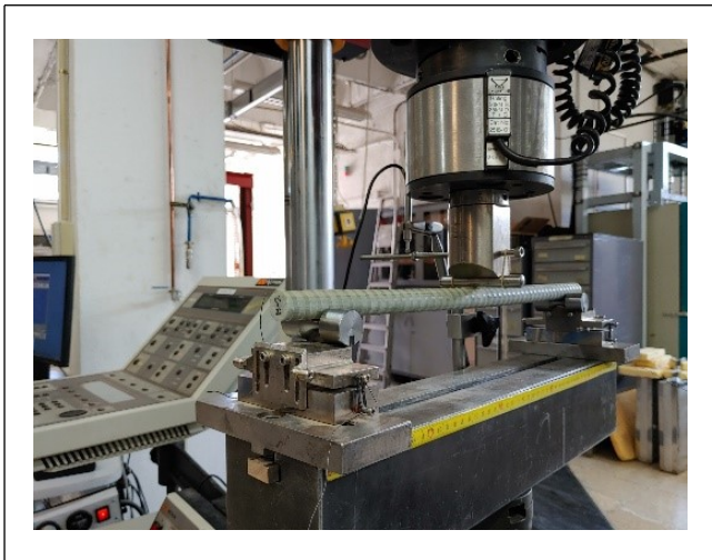
Figure 14. Three-point bending test of FRP rebars performed at UPM
