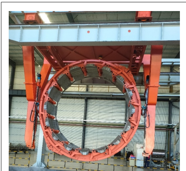
Figure 4. The physical diagram of mine tire unloader machine
