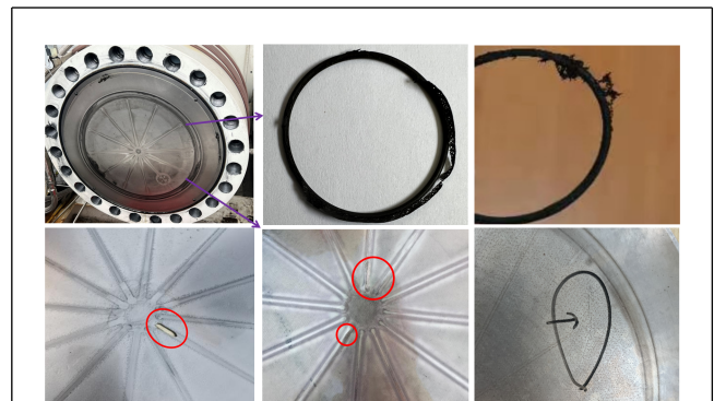
Figure 1. Failure modes of key components for diaphragm compressors
