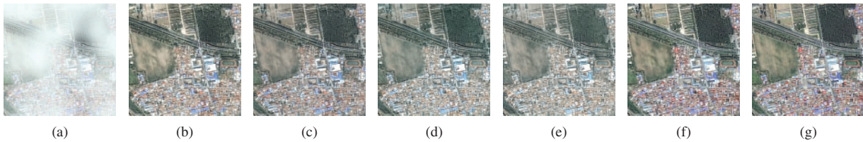
Figure 12: Ablation experimental qualitative evaluations (a) input image (b) without SC-Attention (c) without gater (d) without loss (e) without dense feature fusion (f) URA-net (g) ground truth
