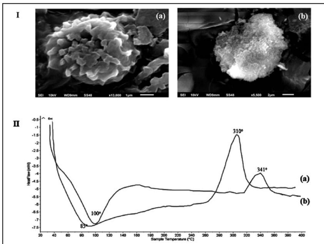
Fig. 5. SEM (I) and DSC thermograms (II) of (a) LLG, and (b) AMLLG.
