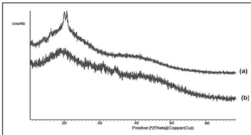
Fig. 4. XRD analysis of (a) LLG, and (b) AMLLG.
