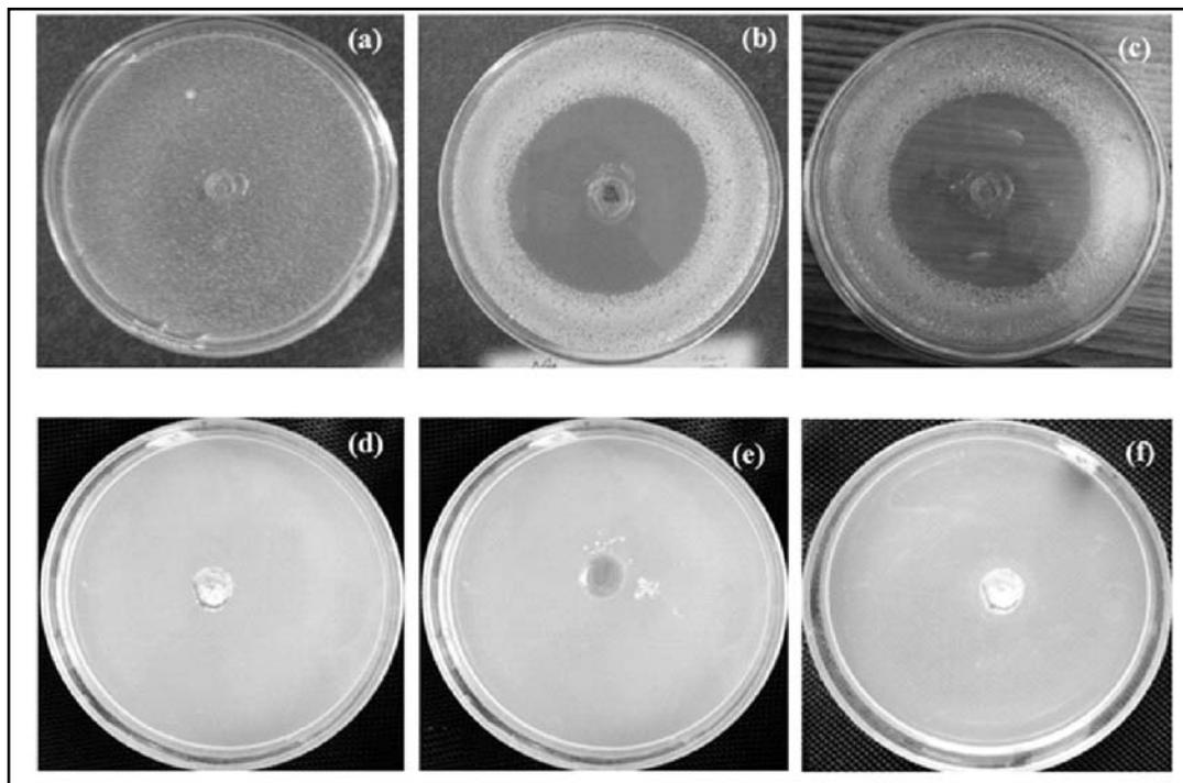
Fig. 8. Antimicrobial properties of (a) LLG (*E. coli*), (b) aminated LLG(*E. coli*), (c) chitosan (*E. coli*), (d) LLG (*S. aureus*), (e) AMLLG (*S. aureus*), and (f) chitosan (*S. aureus*).
