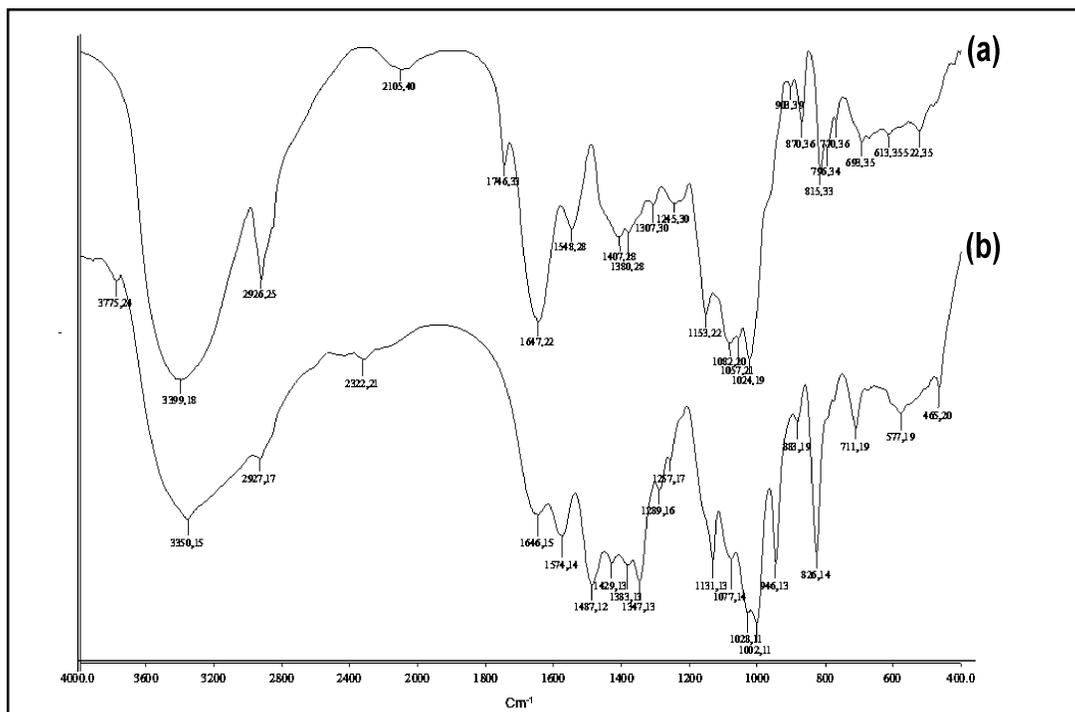
Fig. 3. FTIR spectra of (a) LLG, and (b) AMLLG.
