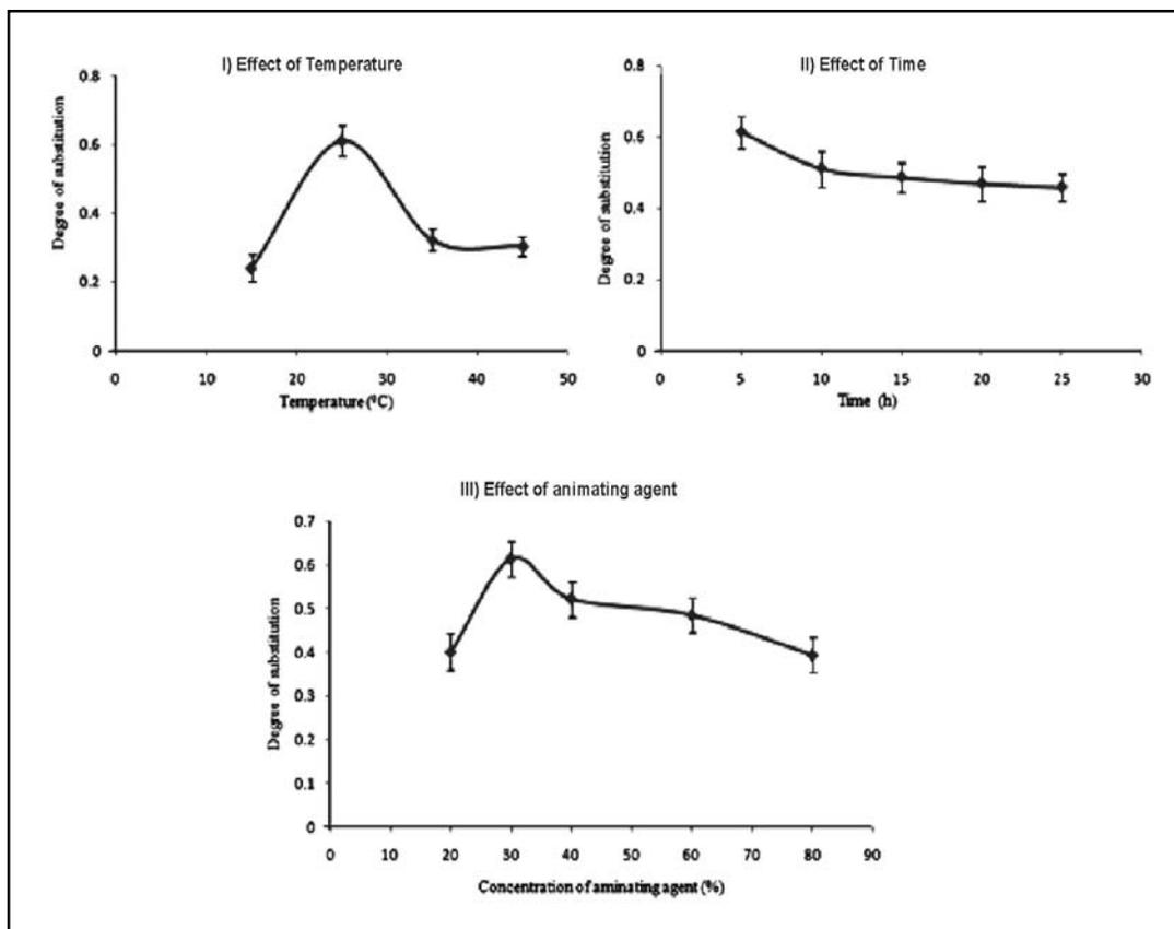
Fig. 2. Effect of (a) temperature, (b) time, and (c) concentration of aminating agent on degree of substitution.
