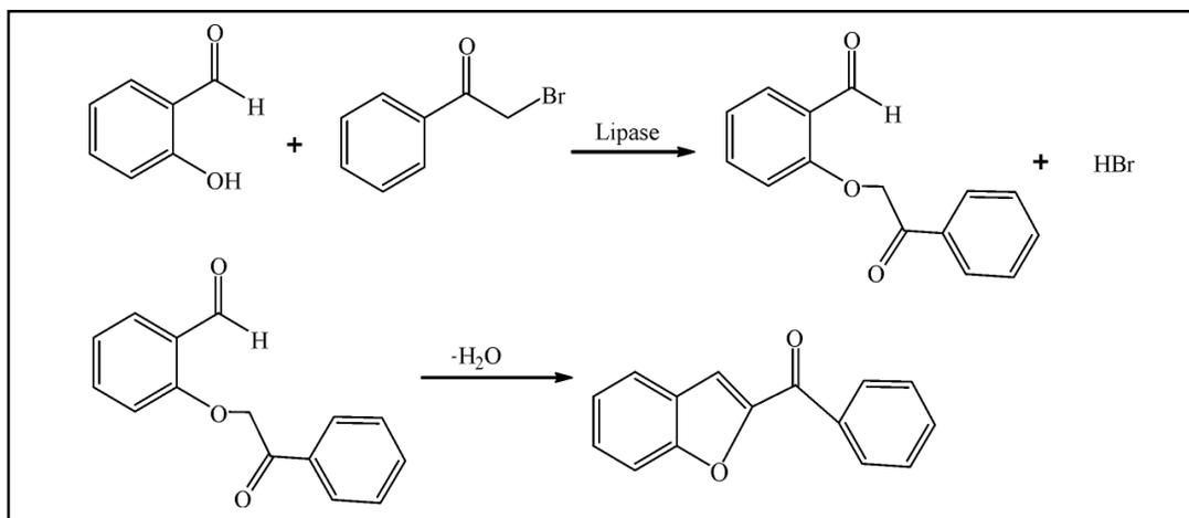
Fig. 3. The specifically reaction process of Rap-Stoermer reaction
