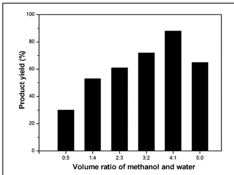
Fig. 5. Effect of volume ratio of methanol and water on product yield
