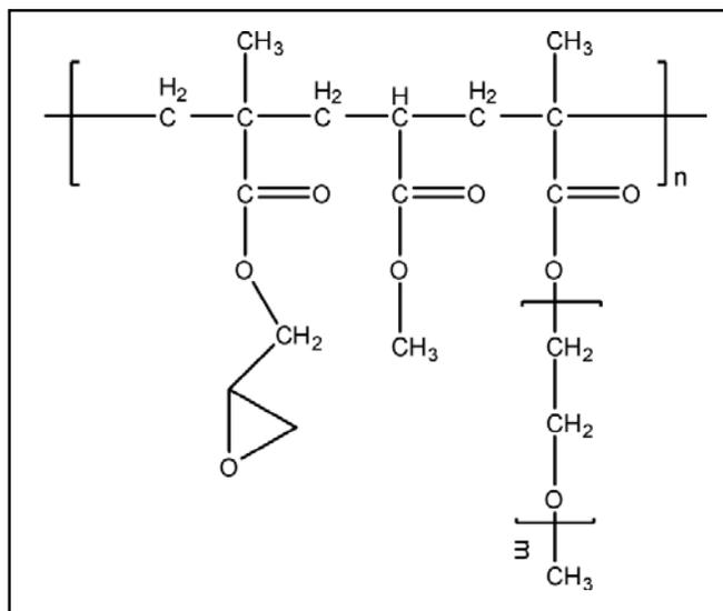
Fig. 1. Chemical structure of P(GMA-co-MA)-g-PEO
