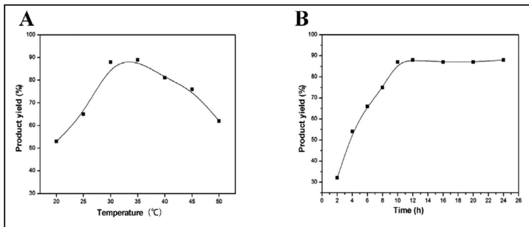
Fig. 7. Effect of (A) reaction temperature and (B) reaction time on product yield
