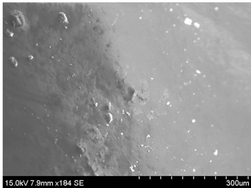
Fig. 3b SEM image of 0.9 wt % electrostatic charged MWCNT
