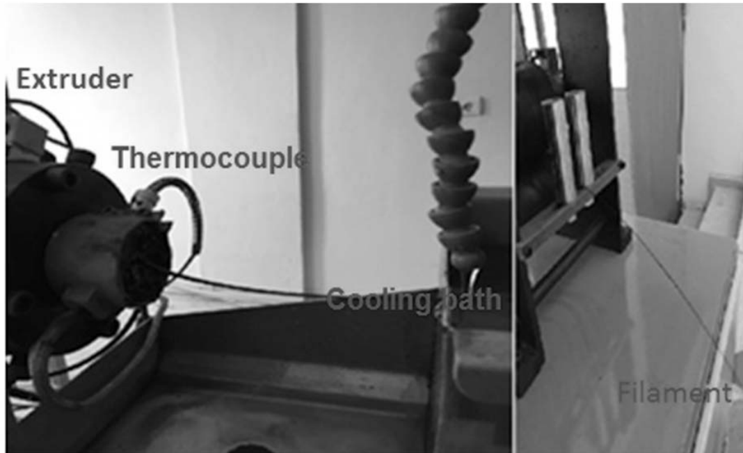
Fig. 2. The extrusion process setup for the ABS-GDM filaments manufacture.
