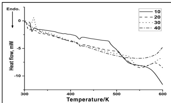
Figure 2. DSC curves for EBHBC-DDM at 5, 10, 15, and 20°C min<sup>-1</sup> heating rates in a nitrogen atmosphere.
