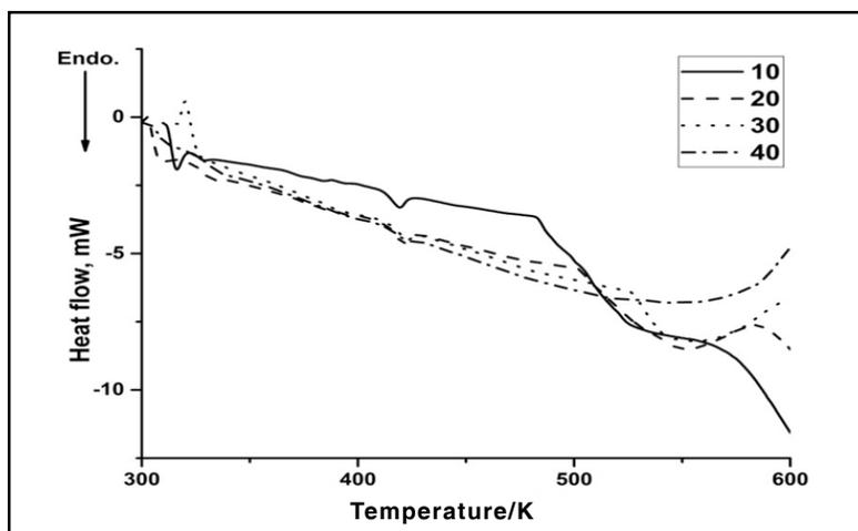
Figure 1. DSC curves for EBHBC at 5, 10, 15, and 20°C min<sup>-1</sup> heating rates in a nitrogen atmosphere.
