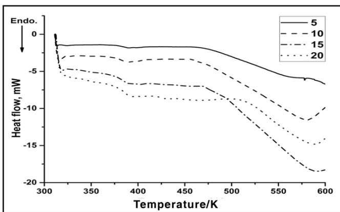
Figure 4. DSC curves for EBHBC-THPA at 5, 10, 15, and 20°C min<sup>-1</sup> heating rates in a nitrogen atmosphere.
