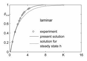
Fig. 4 Thin plate transient temperature and comparison to measurements. Laminar flow.
