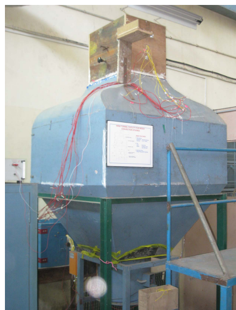
Fig. 3 Schematic of the wind tunnel used for the experiments
