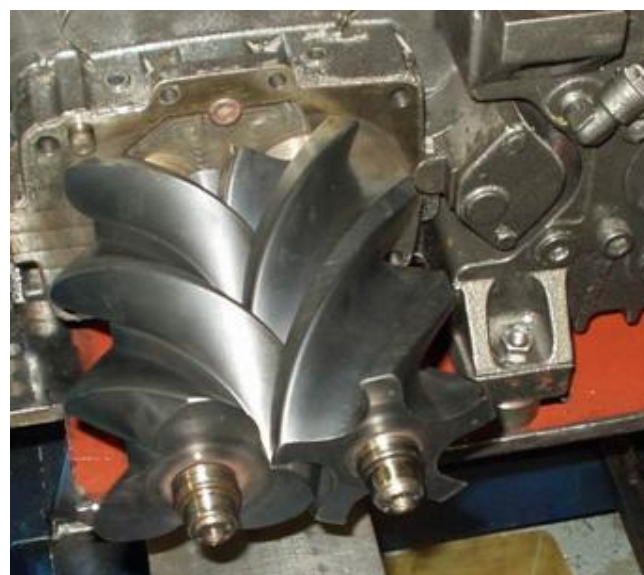
Fig. 8 Compressor rotors, housing removed
