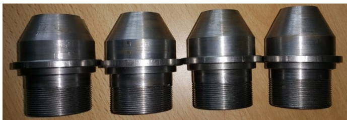
Fig. 4 The photographs of control valves with different throttle diameter(in comparison form) used in the tests
