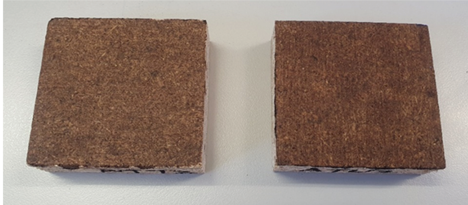
Figure 1: Particleboard panels coated with ATT (left), and with ATU (right)
