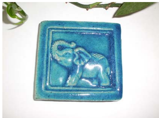
Fig. 5 Glazed tile heated by the catalytic combustion furnace
