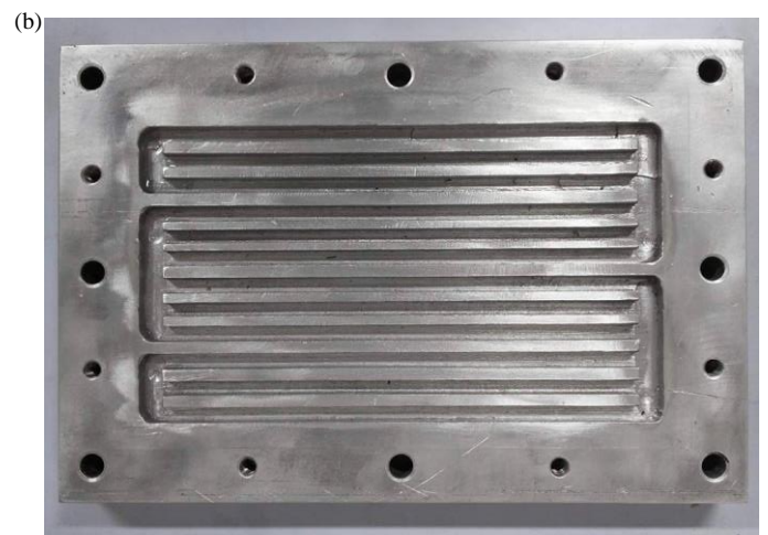
(b) Photograph of the aluminum plate-fin heat sinks
