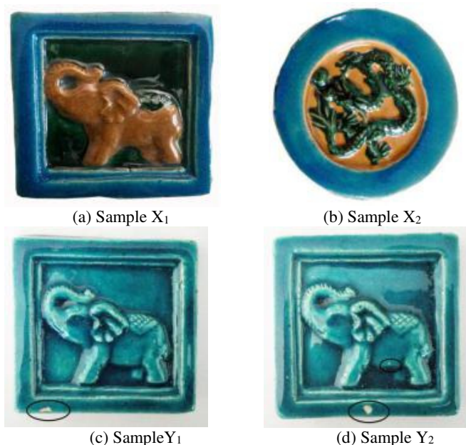
Fig. 5 Views of glazed tile tested to frost resistance
