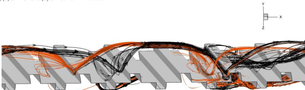
Fig. 14 Longitudinal vortex flow of the heat exchanger tube equipped with the inclined wavy surface for \alpha = 60^\circ at Re = 6000 .
