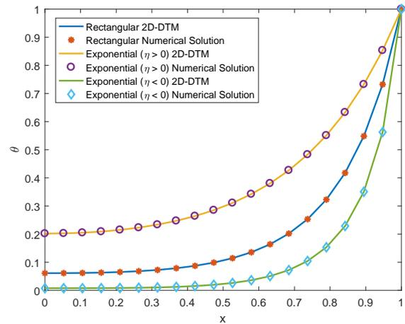
Fig. 2. Temperature distribution in differing fin profiles.
