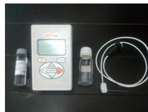
**Fig. 3** KD2 Pro hot wire meter of thermal conductivity.
