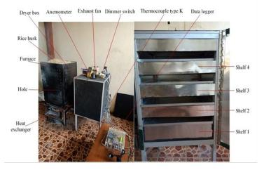
Fig. 2 Testing of jackfruit dodol samples on rice husk biomass dryer
