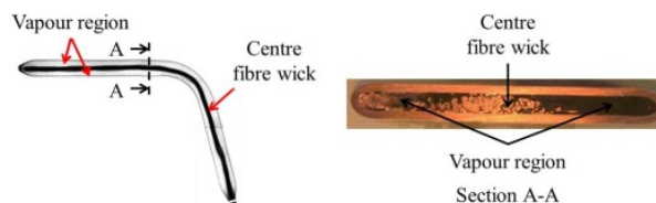
Fig. 7 X-ray image of the flattened heat pipe and cross sectional cut. Some stray fibers are seen in the cross sectional cut – these were present due to the cutting procedure only as can be confirmed by the x-ray image.
