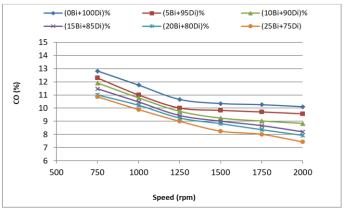
Fig. 6 Effects of different biodiesel rates on CO emissions at different speeds.
