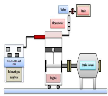
Fig. 1 Experimental setup of the rig.
