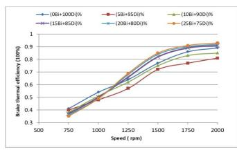
Fig. 4 The effects of biodiesel rate on Nbth at different speeds.
