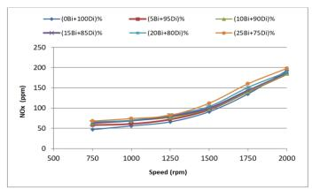
Fig. 8 Effects of different biodiesel rates on NOx emissions at different speeds.
