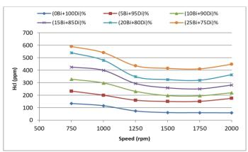
Fig. 7 Effects of different biodiesel rates on Hcl emissions at different speeds.
