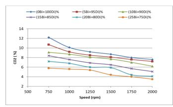
Fig. 5 Effects of different biodiesel rates on CO2 emissions at different speeds.
