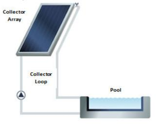
Fig. 5 Proposed SWHS for outdoor Swimming Pool in TSOL® Simulation Tool
