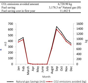
Fig.13 CO<sub>2</sub> emissions amount avoided vs. amount saving of natural gas of SWHS proposed
