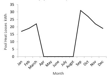
Fig. 11 Monthly heat losses of the pool of SWHS proposed
