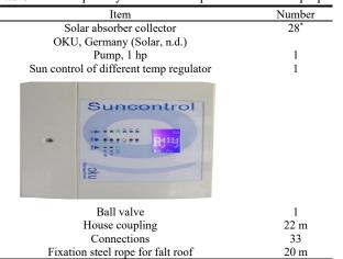
\* Calculation of pool surface: 13 m length  $\times$  4 m width = 52 m<sup>2</sup>. For pool without cover; we recommended approx 60% of the pool surface as absorber surface.
