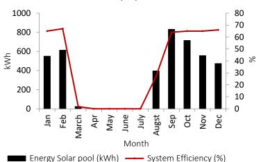
Fig. 10: Solar energy contribution to swimming pool vs. SWHS proposed efficiency
