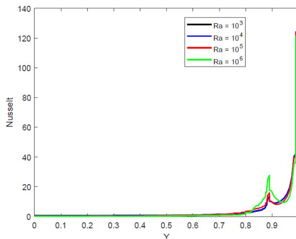
**Fig. 5:** Deviation of Nusselt number along the vertical section with rectangular block at the Top of the cavity.
