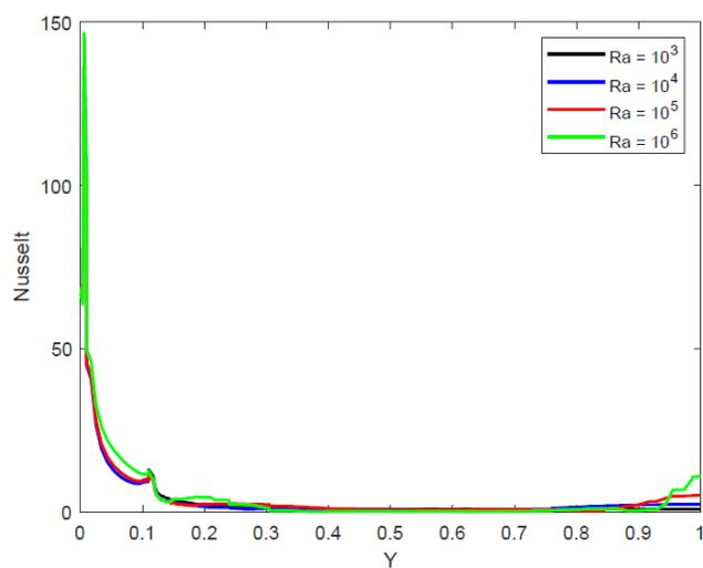
**Fig. 7:** Deviation of Nusselt number along the vertical section with rectangular block at the Bottom of the cavity
