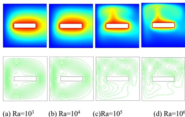
**Fig. 3:** Isotherms (up) and Streamlines (down) of heated block located at the center of the cavity for (a)  $Ra=10^3$  (b)  $Ra=10^4$  (c)  $Ra=10^5$  (d)  $Ra=10^6$
