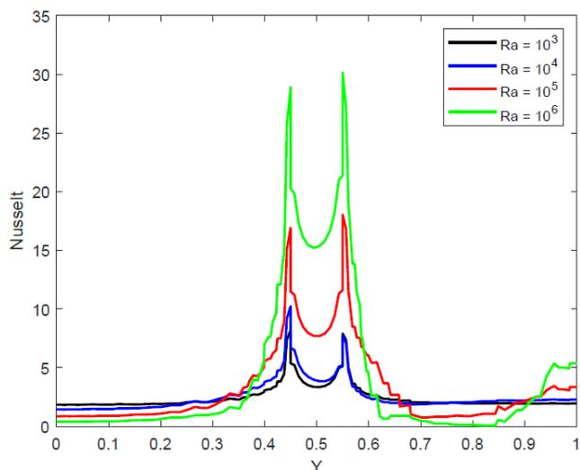
**Fig. 6:** Deviation of Nusselt along the vertical section with rectangular block at the Middle of the cavity
