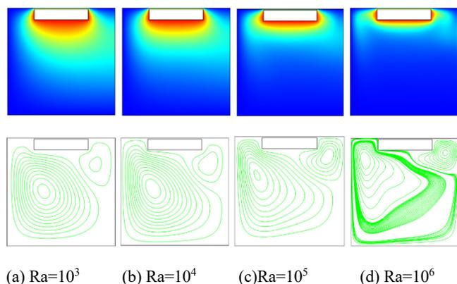
**Fig. 2:** Isotherms (up) and Streamlines (down) of heated block located at the top of the cavity for (a)  $Ra=10^3$  (b)  $Ra=10^4$  (c)  $Ra=10^5$  (d)  $Ra=10^6$
