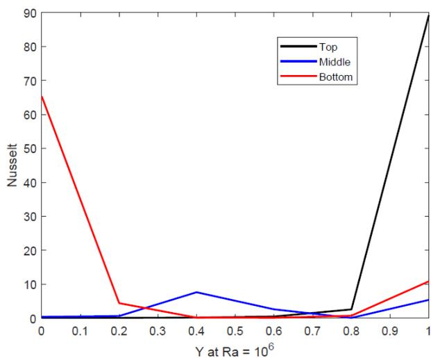
**Fig. 11:** Deviation of Nusselt number for the three position Top, Center and Bottom at  $Ra=10^6$  within the cavity
