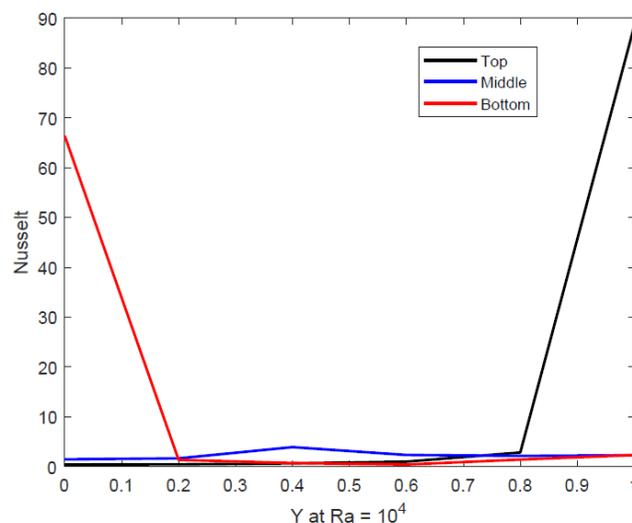
**Fig. 9:** Deviation of Nusselt number for the three position Top, Center and Bottom at  $Ra=10^4$  within the cavity
