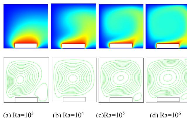
**Fig. 4:** Isotherms (up) and Streamlines (down) of heated block located at the bottom of the cavity for (a)  $Ra=10^3$  (b)  $Ra=10^4$  (c)  $Ra=10^5$  (d)  $Ra=10^6$
