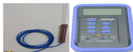
(b) Digital and Cable Thermocouple
