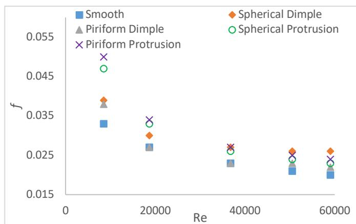
**Fig. 11.** Friction factors of the test channels
