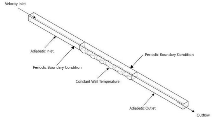
**Fig. 3.** Boundary conditions for the dimpled channel
