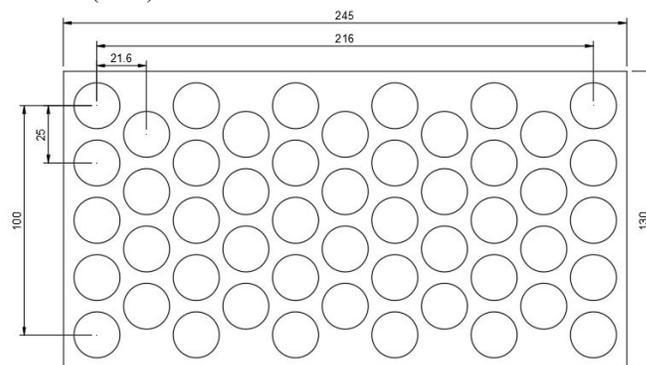
**Fig. 1.** Arrangement of dimples/protrusions in the test section
