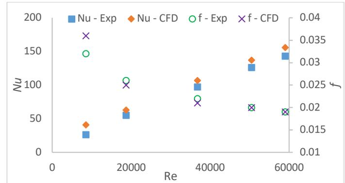
Fig. 5: Nusselt number and friction factor obtained with experimental data
