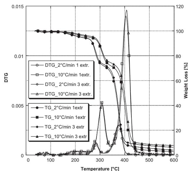
**Figure 1** TGA curves of pure Mater-Bi® after one and three extrusion steps at different heating rates.
