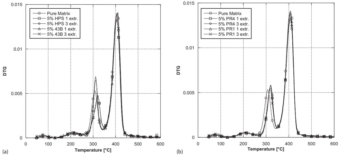
**Figure 2** Comparison of thermal degradation DTG curves at  $10^{\circ}\text{C min}^{-1}$  of the pure matrix with (a) Montmorillonite-reinforced nano-biocomposites, and (b) Sepiolite-reinforced nano-biocomposites.
