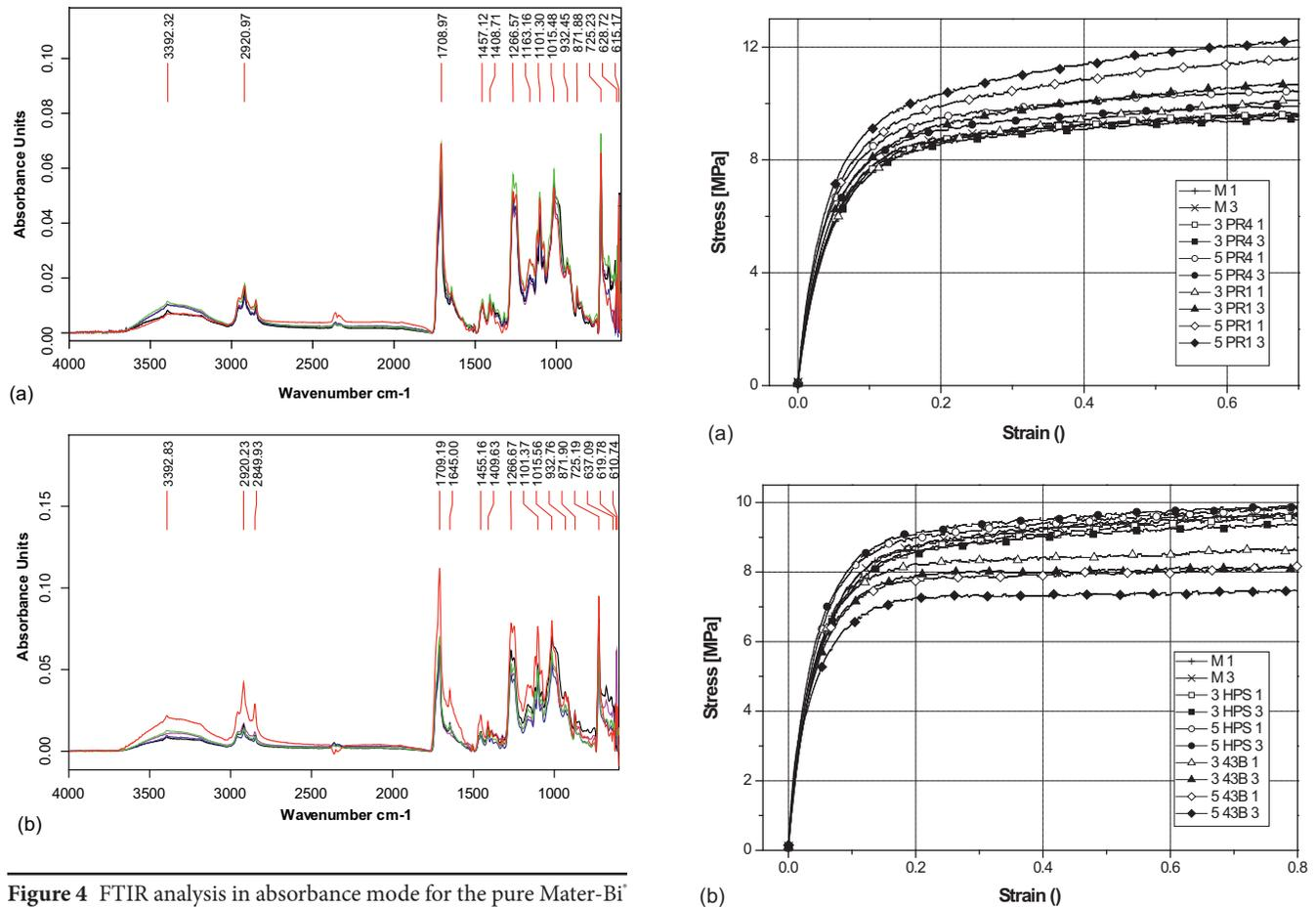
**Figure 4** FTIR analysis in absorbance mode for the pure Mater-Bi matrix (red) and nano-biocomposites with pure sepiolite 3 wt% (blue), pure sepiolite 5 wt% (magenta), modified sepiolite 3 wt% (green), modified sepiolite 5 wt% (black); (a) after one extrusion, (b) after three extrusions.
