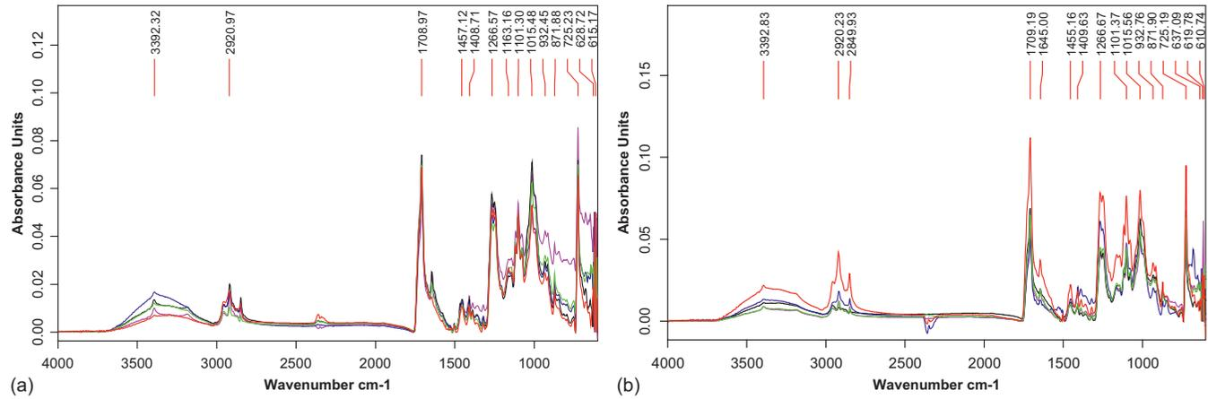
**Figure 3** FTIR analysis in absorbance mode for the pure Mater-Bi matrix (red) and nano-biocomposites with MMT 3 wt% (blue), MMT 5 wt% (magenta), modified MMT 3 wt% (green), and modified MMT 5 wt% (black); (a) after one extrusion, (b) after three extrusions.
