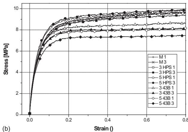
**Figure 5** Stress-strain curves of nano-biocomposites: (a) montmorillonite; (b) sepiolite.
