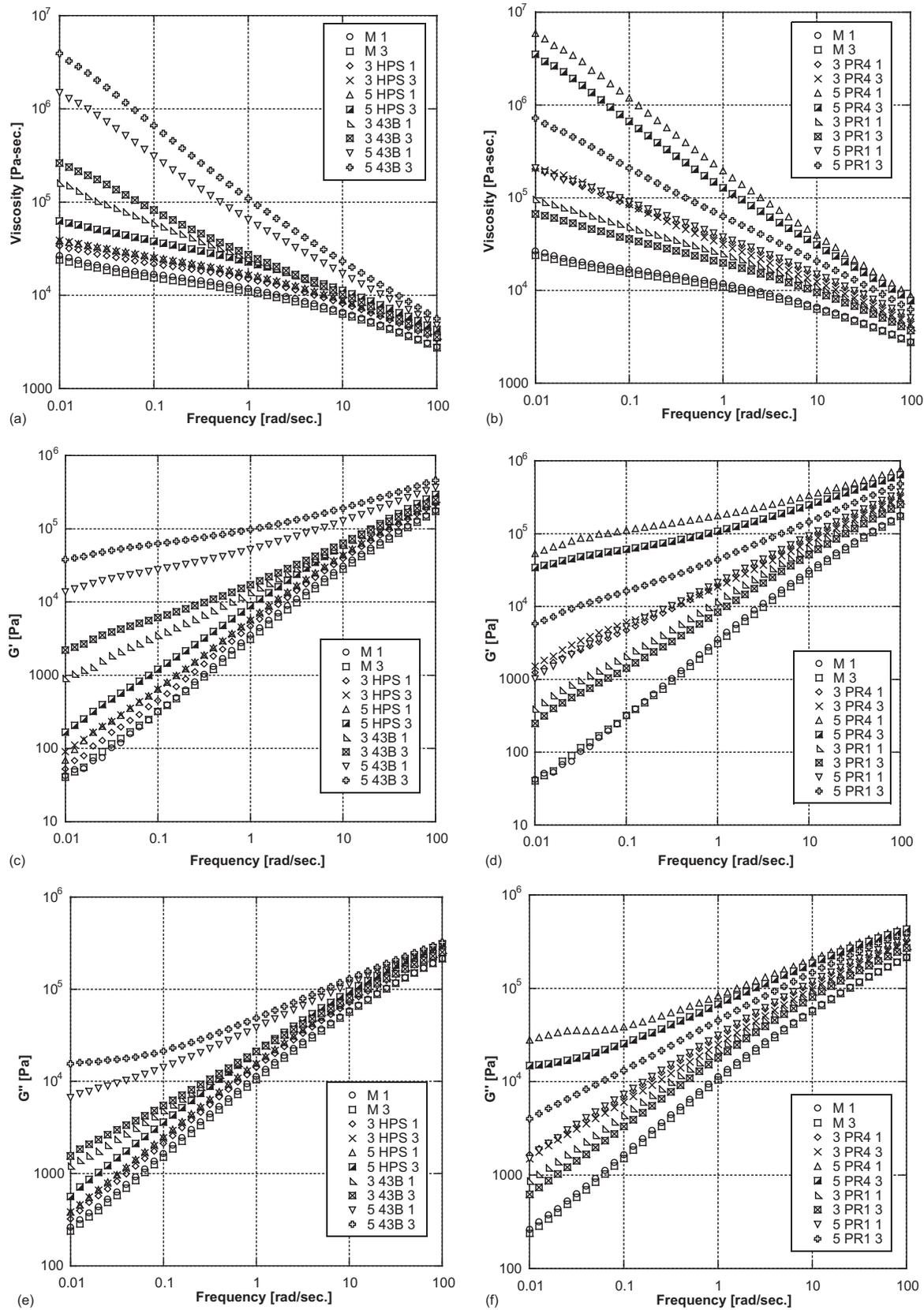
**Figure 7** Complex viscosity, storage modulus ( $G'$ ) and loss modulus ( $G''$ ) of the pure matrix: (a,c,e) MMT filled systems and (b,d,f) Sepiolite filled systems.
