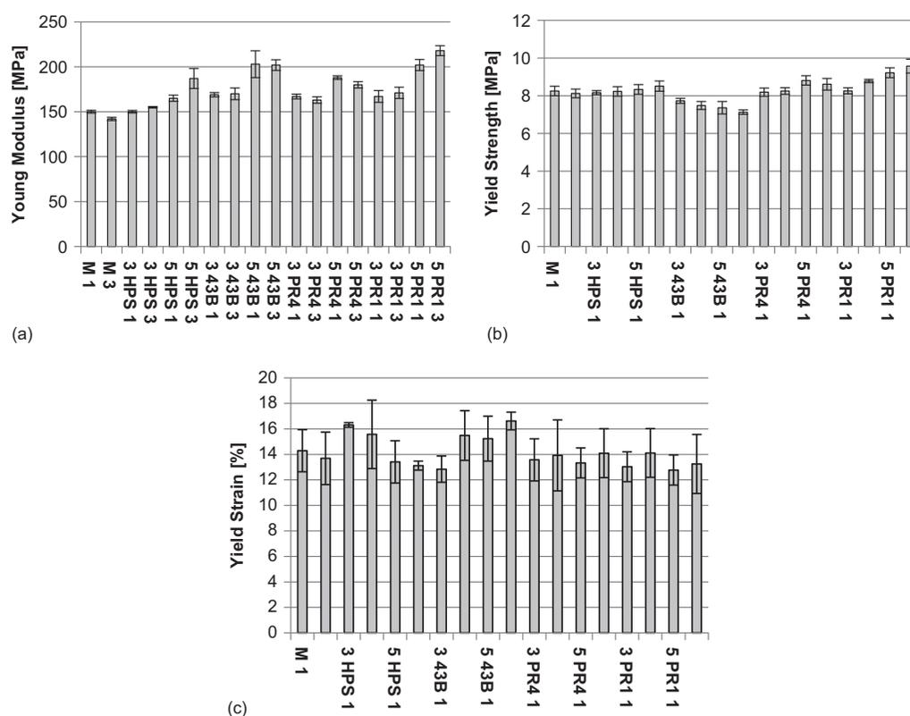
**Figure 6** (a) Elastic modulus, (b) yield strength and (c) yield strain of the nano-biocomposites.
