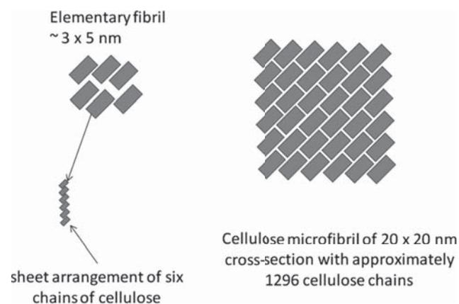
**Figure 1** Sketch of cellulose structures at different levels from cellulose chains to microfibrils.
