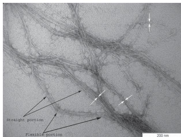
**Figure 4** TEM image of MFC produced from larger fibrils showing rigid and flexible regions.
