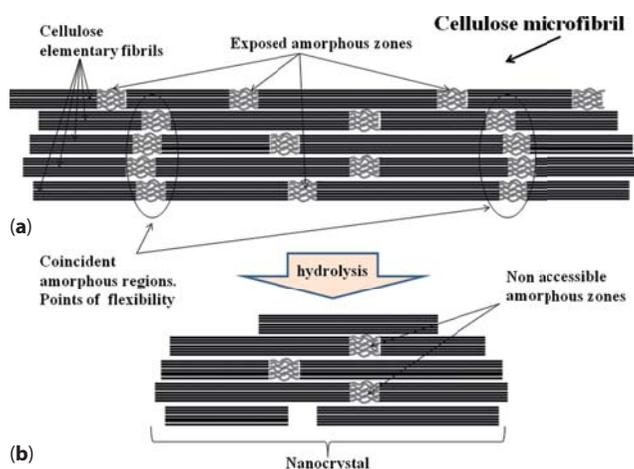
**Figure 6** Schematic model for cellulose microfibrils and their hydrolysis product; (a) before hydrolysis and (b) after hydrolysis of the most accessible amorphous cellulose.
