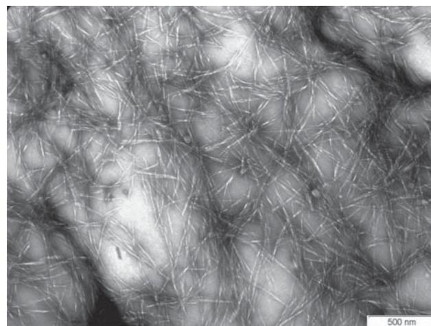
fibrils are aligned in the axial direction and are being detached from the microfibril. They show very regular dimensions of an approximately 5 nm diameter.
