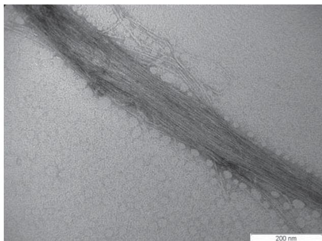
**Figure 3** TEM image of MFC formed by the self-assembly of elementary microfibrils.
