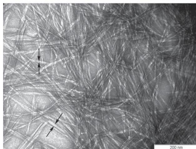
**Figure 5** TEM image of CNC produced from eucalyptus wood pulp.
