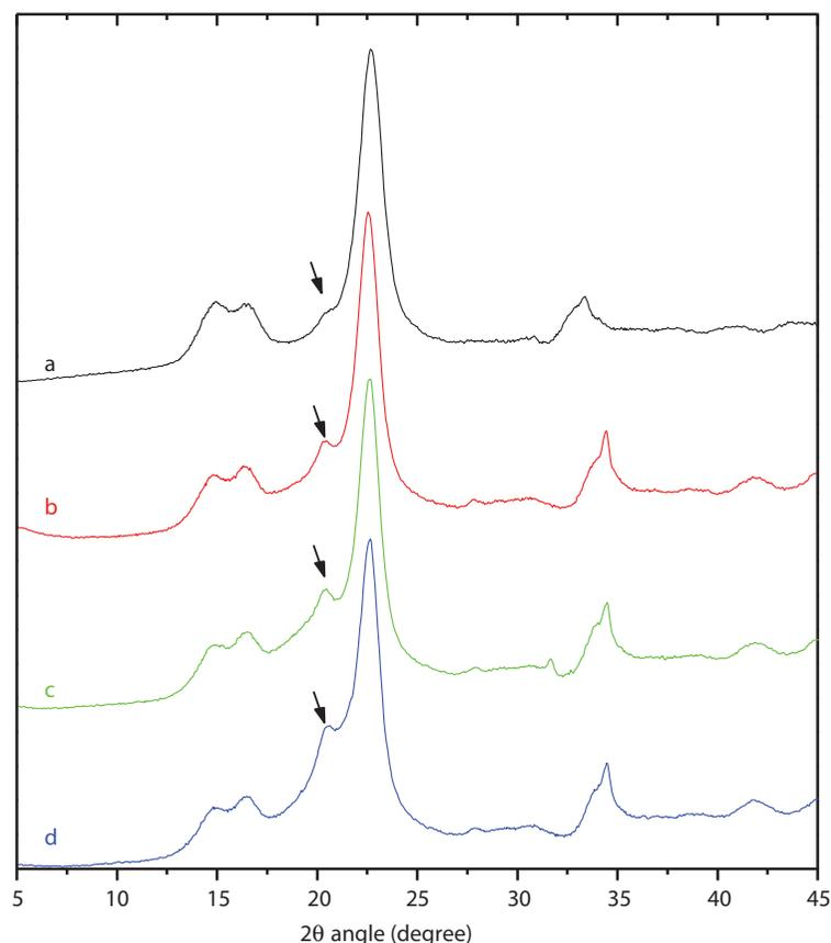
**Figure 6** X-ray diffraction patterns for unmodified ramie cellulose nanocrystals (a) and modified with hexanoyl chloride (b), lauroyl chloride (c) and stearoyl chloride (d).
