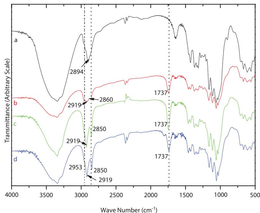
**Figure 4** FTIR spectra (KBr pellets) of unmodified ramie cellulose nanocrystals (a) and modified with hexanoyl chloride (b), lauroyl chloride (c) and stearoyl chloride (d).
