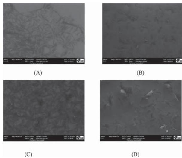
**Figure 5** FEG-SEM of unmodified ramie cellulose nanocrystals (a) and modified with hexanoyl chloride (b), lauroyl chloride (c) and stearoyl chloride (d).
