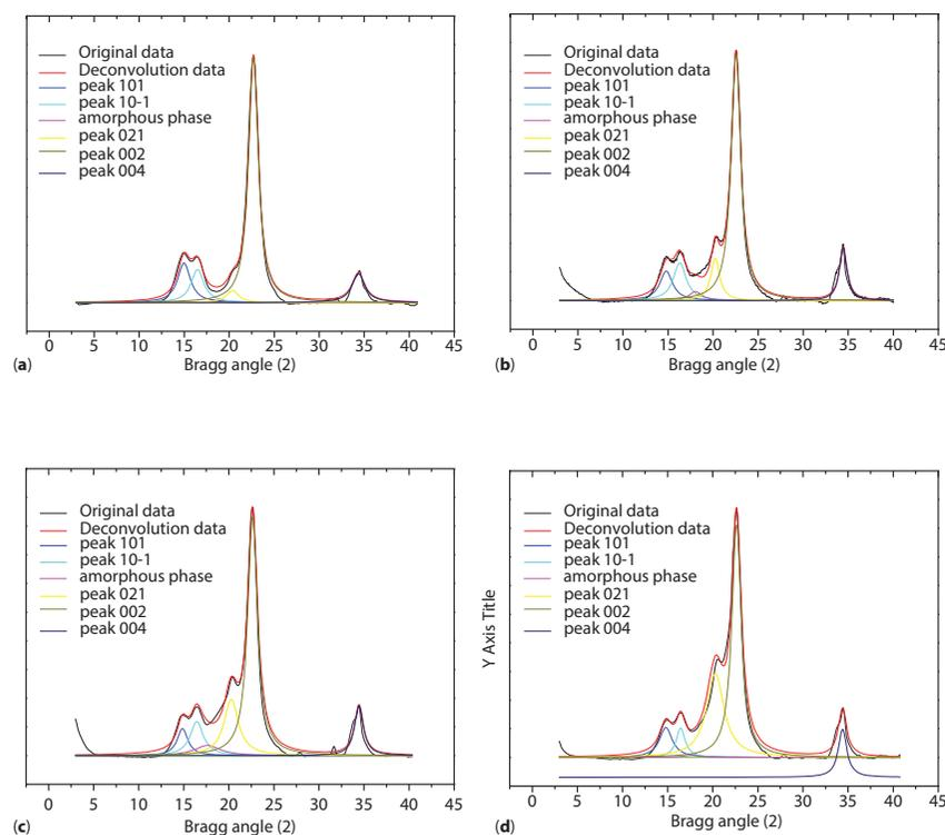
**Figure 7** X-ray diffraction patterns and peak deconvolution for unmodified ramie cellulose nanocrystals (a) and modified with hexanoyl chloride (b), lauroyl chloride (c) and stearoyl chloride (d).
