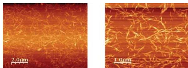
Figure 1 Atomic force micrograph of ramie cellulose nanocrystals.
