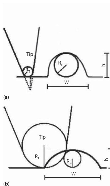
Figure 2 Illustration of lateral enlargement of AFM imaging in the case where only the tip radius curvature interacts with the sample (a) and for the case where both the tip apex and walls interact with the sample (b) [24].
