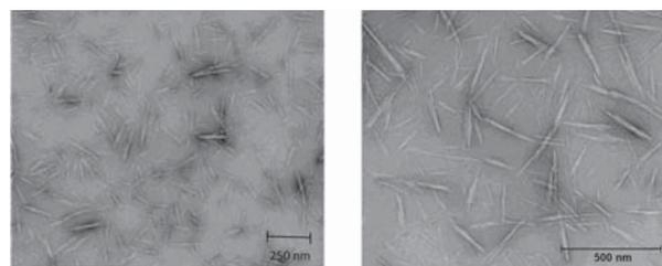
Figure 3 Transmission electron micrographs of ramie cellulose nanocrystals.
