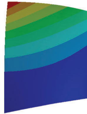
Figure 4: First modal shape of the blade
