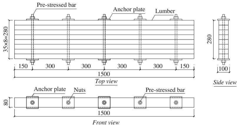
**Figure 2:** Diagrams for P600-S300 specimens (dimensions in mm)
