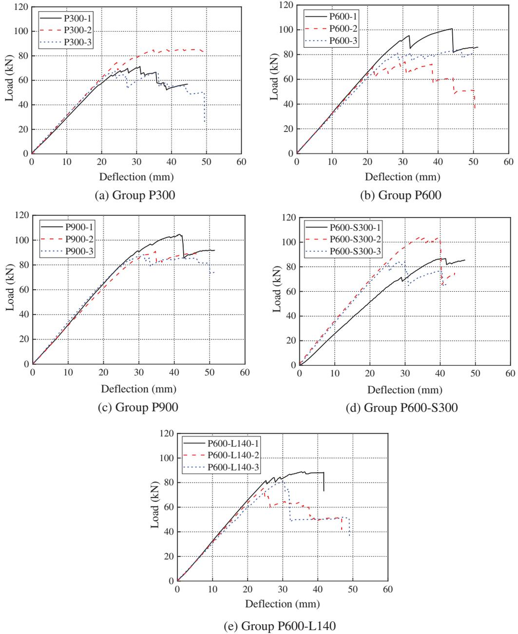
**Figure 7:** Load-deflection curves of SLT specimens
