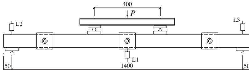
**Figure 4:** Test setup (dimensions in mm)
