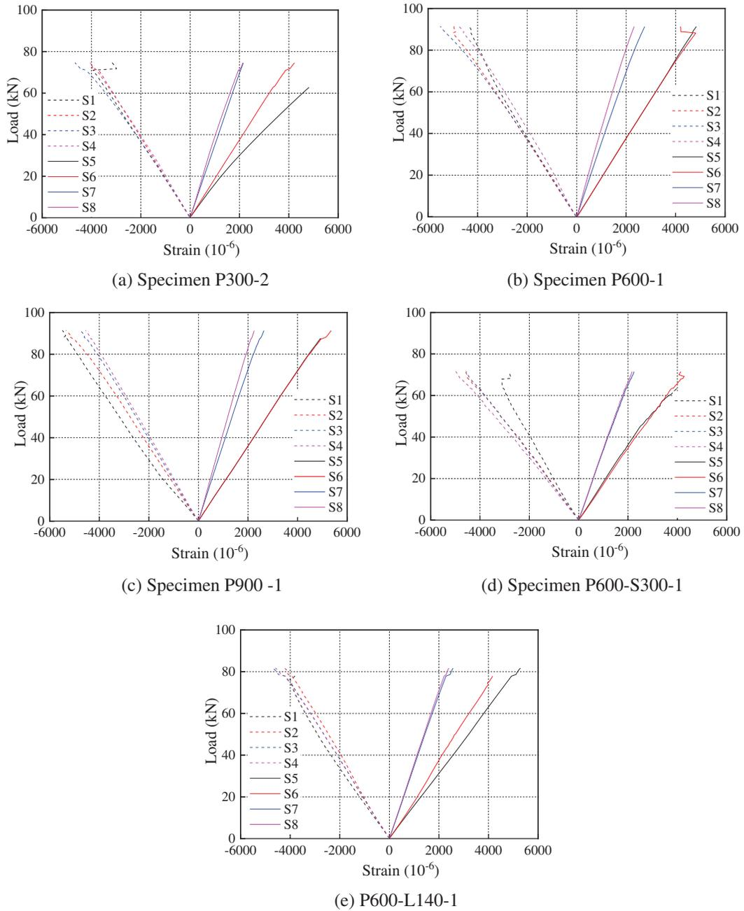
**Figure 8:** Load-strain curves of SLT specimens
