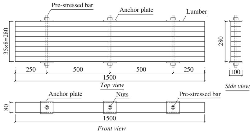
**Figure 1:** Diagrams for P300, P600, and P900 specimens (dimensions in mm)
