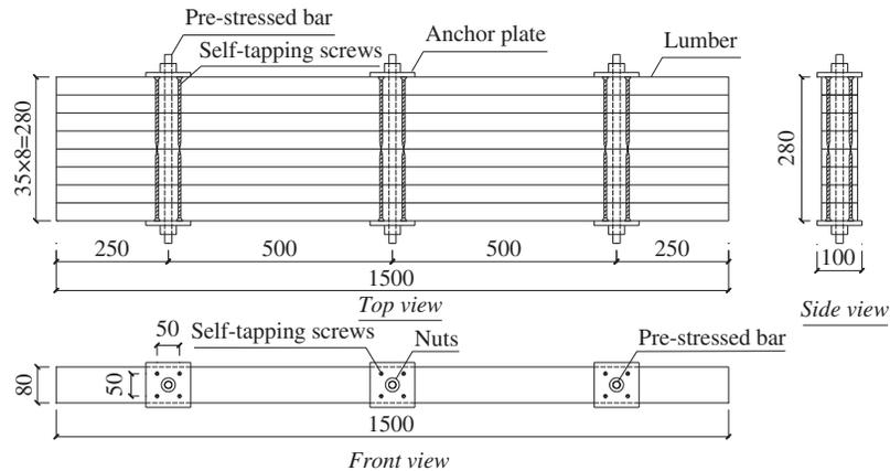
**Figure 3:** Diagrams for P600-L140 specimens (dimensions in mm)
