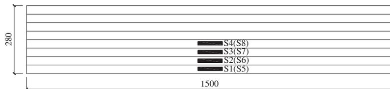
**Figure 5:** Layout of strain gauges on SLT specimens (dimensions in mm)
