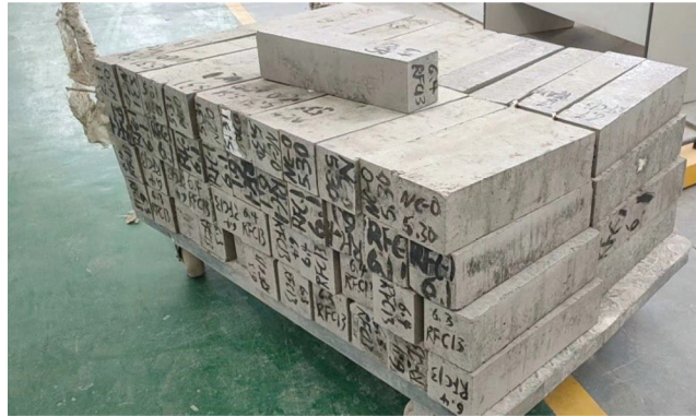
Figure 3: 100 mm × 100 mm × 400 mm sample diagram
