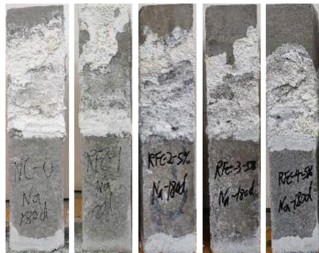
Figure 5: Corrosion morphology of RPC in \text{Na}_2\text{SO}_4 solution Note: The replacement rate is 0%, 10%, 20%, 30%, and 40% from left to right.
