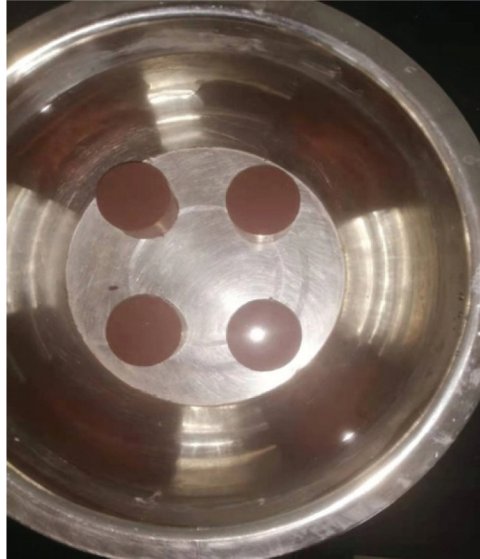
Figure 3: Baking-free samples in a water tank during the water absorption test
