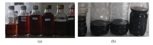
**Figure 3:** LDPE plastic pyrolysis liquid product: (a) without catalyst and (b) with activated natural zeolite catalyst
