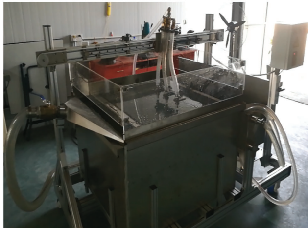
Figure 2: Scour test bench
