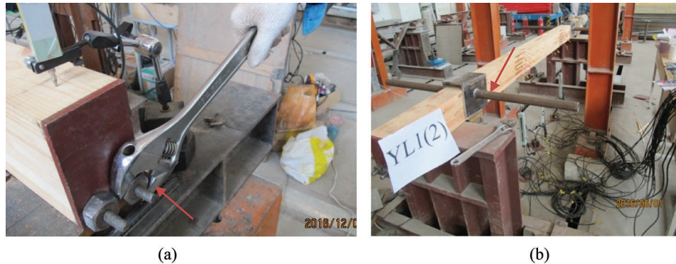
Figure 5: Application of the prestress. (a) Screw nut. (b) Auxiliary device
