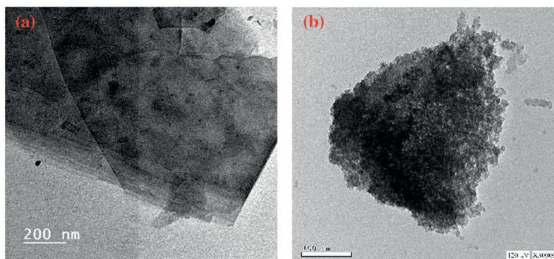
**Figure 2:** TEM of (a) GO and (b) MGO
