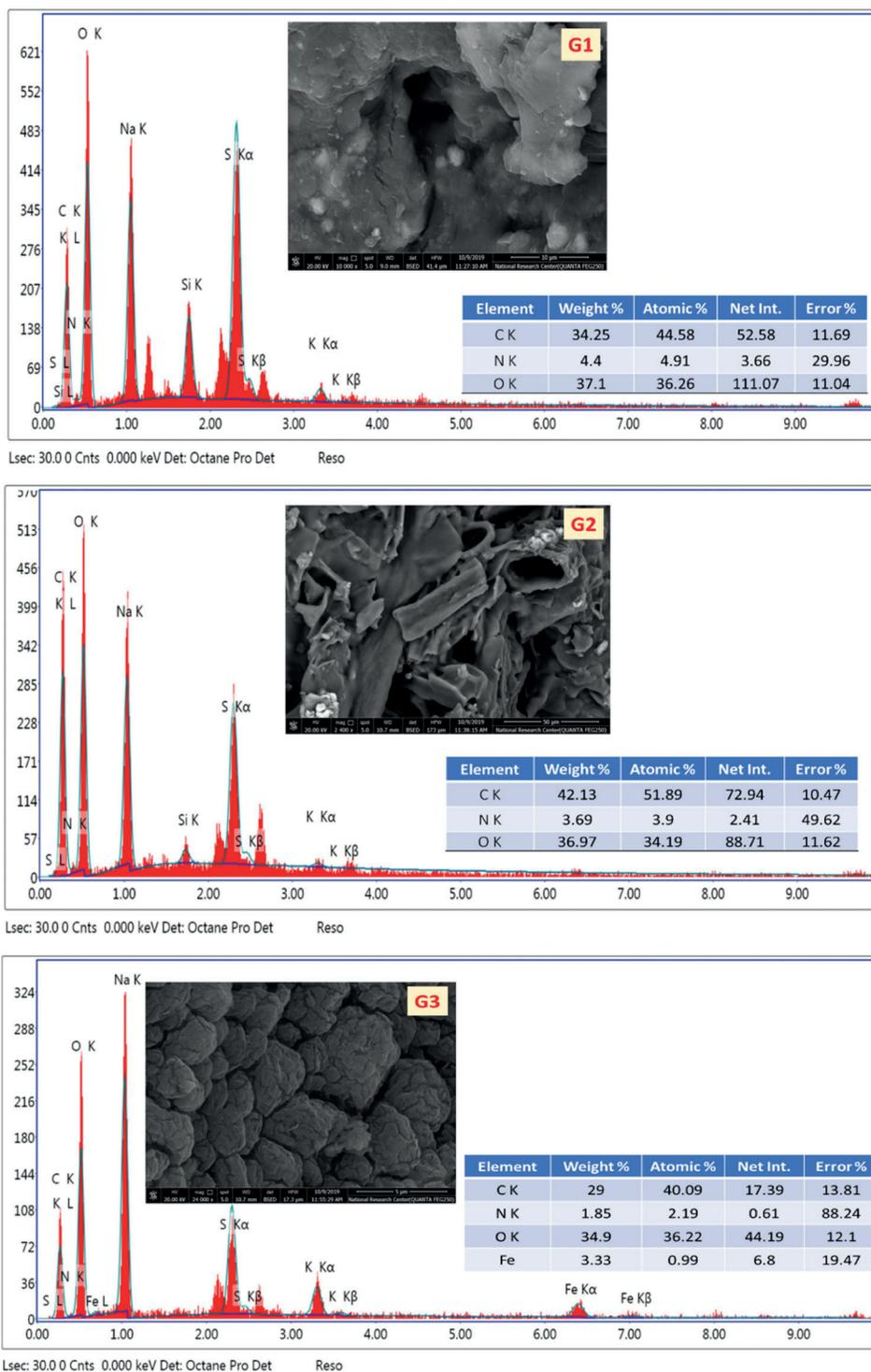
**Figure 3:** Digital photos, SEM and EDX analysis of GO, CMC, MGO, G1, G2, and G3
