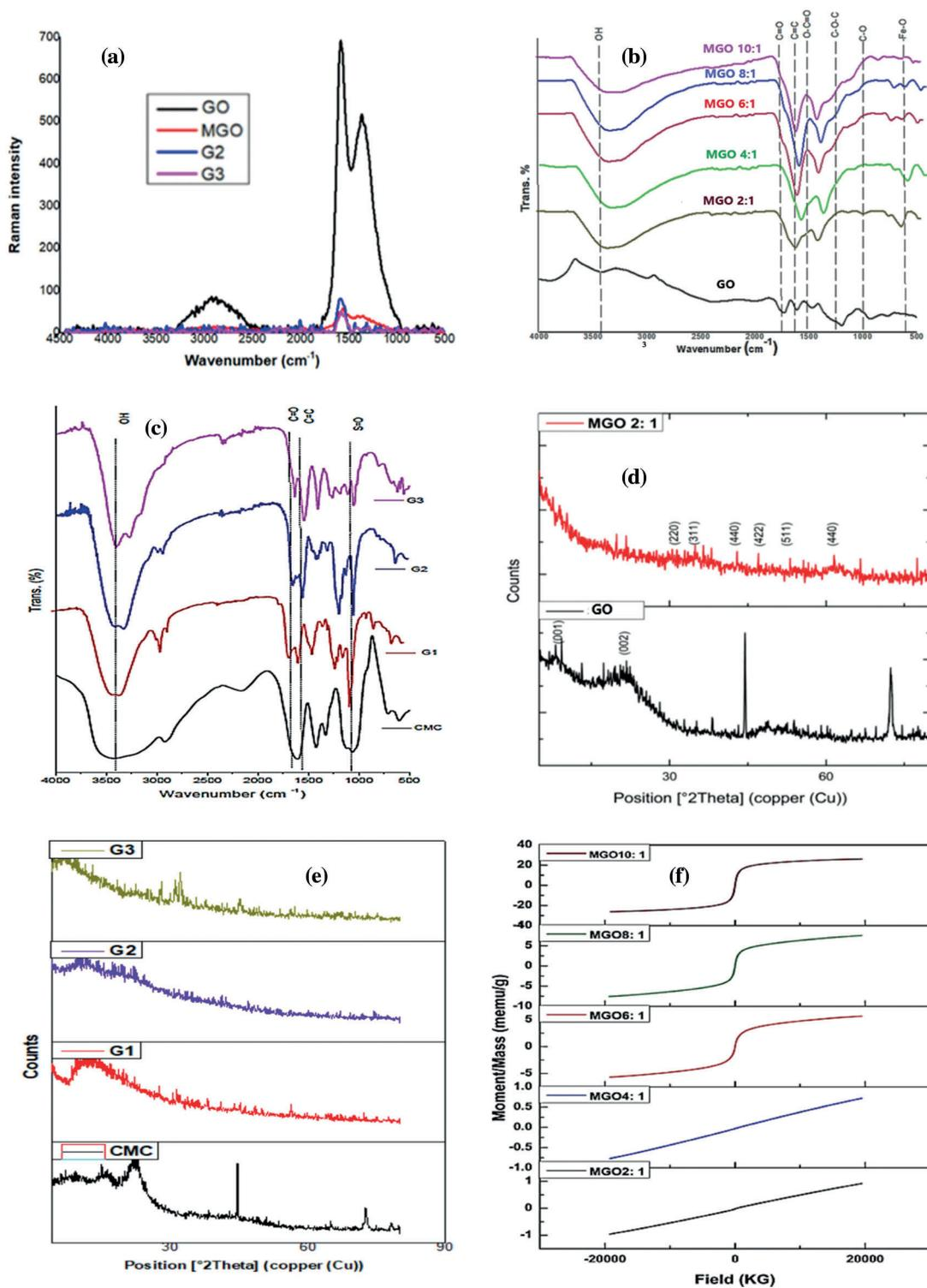
**Figure 1:** (a) Raman spectra of GO, MGO, G2, and G3. (b) FT-IR spectra of GO and MGO. (c) FT-IR spectra of CMC, G1, G2, and G3. (d) XRD patterns of GO and MGO. (e) XRD patterns of CMC, G1, G2, and G3. (f) The magnetic hysteresis curve of MGO nanocomposite
