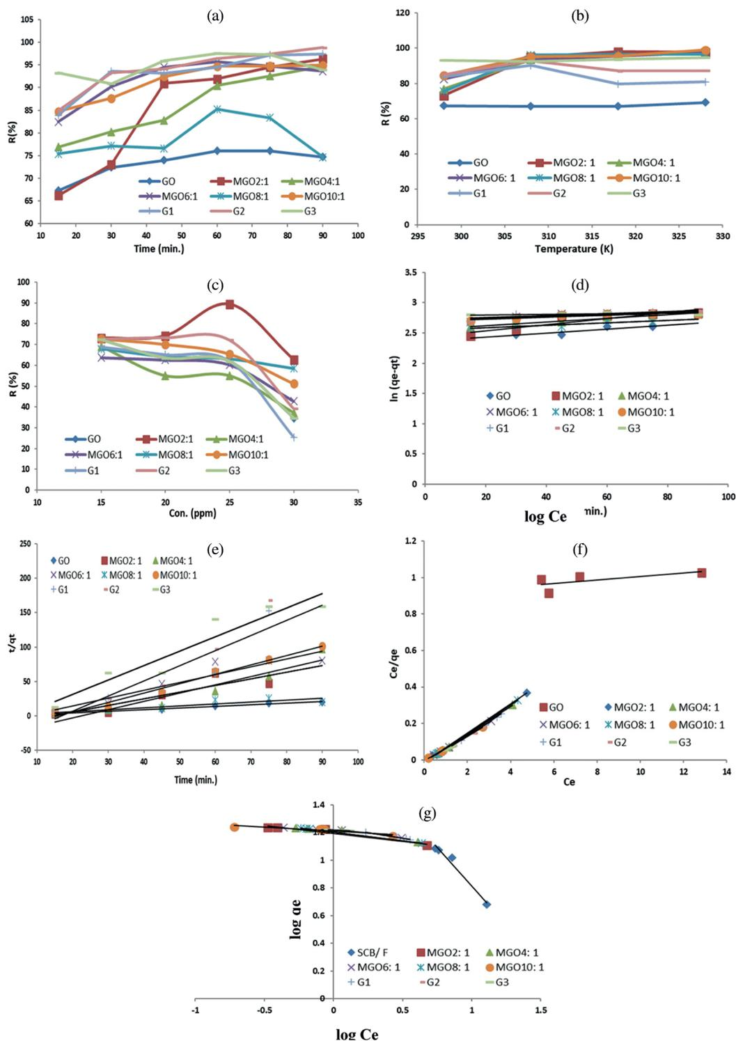
**Figure 5:** Effect of (a) Contact time, (b) Temperature, (c) Ni(II) initial concentration, on Ni(II) adsorption. (d) Kinetics of pseudo first order (e) Kinetics of pseudo second order, (f) Langmuir isotherms, and (g) Freundlich isotherms
