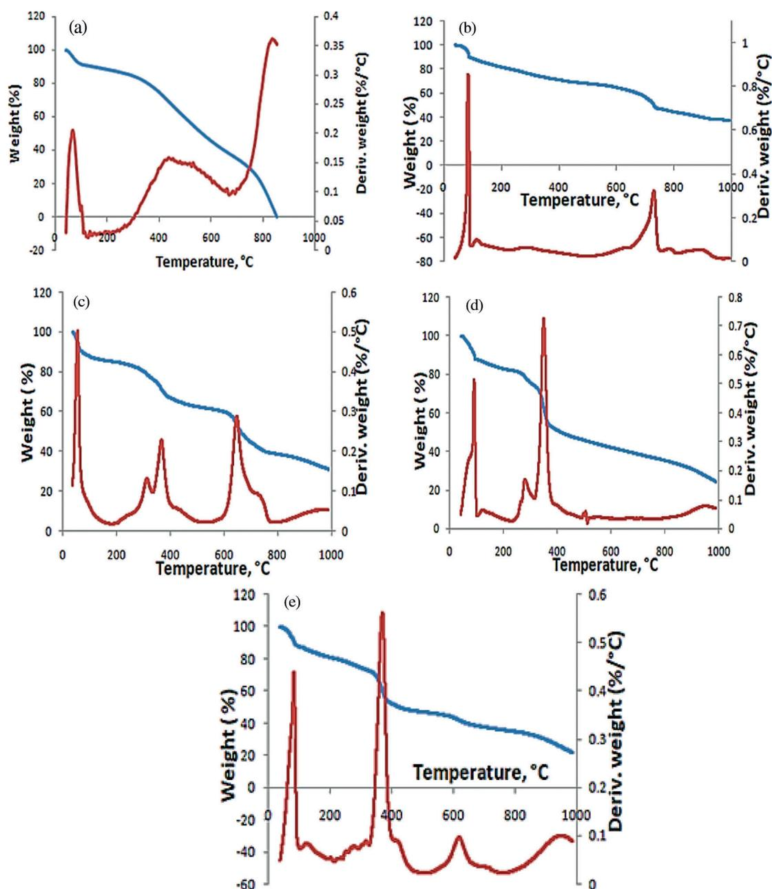
**Figure 4:** TGA and DTA curves of (a) GO, (b) MGO, (c) G1, (d) G2, and (e) G3
