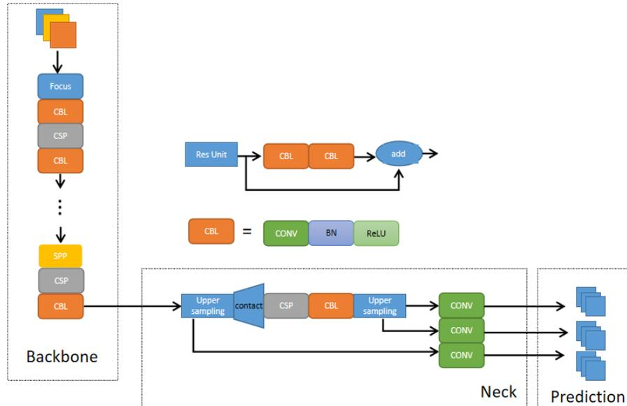
**Figure 1:** The network model structure of YOLOv5
