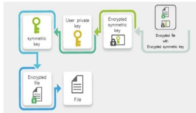
**Figure 12:** Decryption process in integrating two types of algorithms
