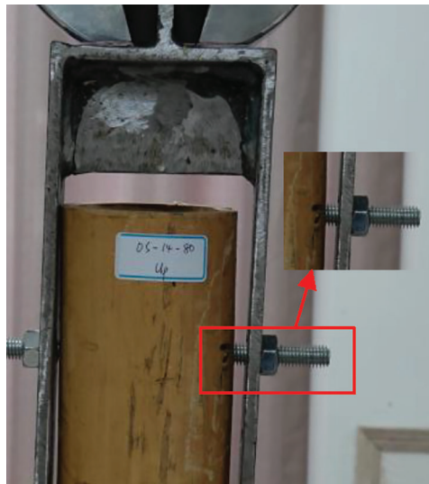
Figure 6: The bolt hole in direct contact with the bamboo
