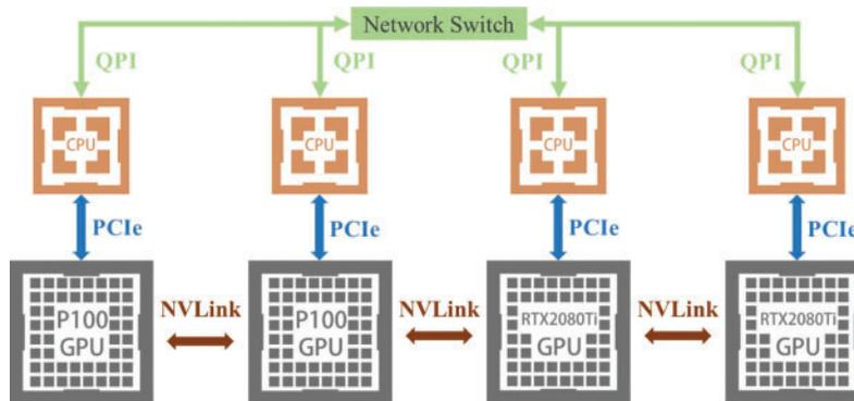
Figure 9: GPU cluster workstation
