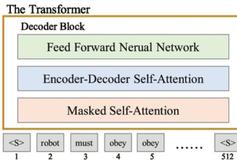
**Figure 2:** GPT-2 decoder architecture
