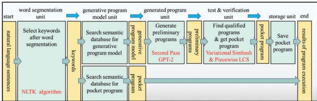
Figure 6: Model use stage architecture diagram
