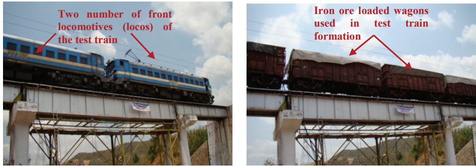
Figure 9: Formation of test train over the steel bridge considered in the present study
