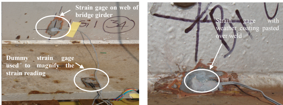
Figure 8: Typical arrangement of strain gages on the flange and the web of the plate girder
