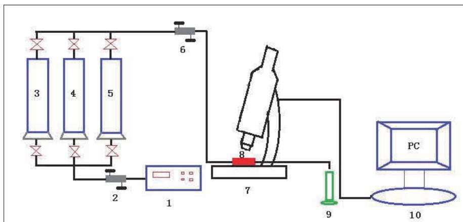
1—High Pressure Syringe Pump 2、6—Triple Valve 3、4、5—Intermediate Container
