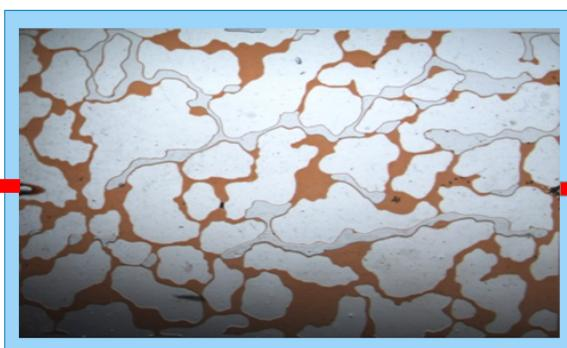
Figure 1: Etched Glass Micro-model
