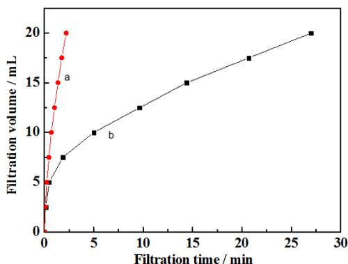
Figure 5: Relationship of filtration volume and filtration time of microspheres dispersed system and HPAM solution (a. HPAM; b. microspheres)
