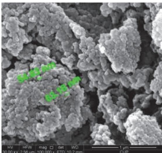
Figure 1: Scanning electron micrograph of crosslink polyacrylamide microspheres.
