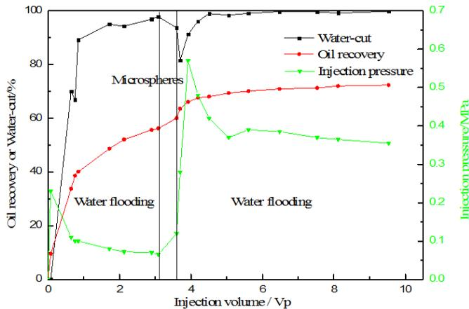
Figure 7: The displacement test curve of heterogeneous double-tube sand pack model.
