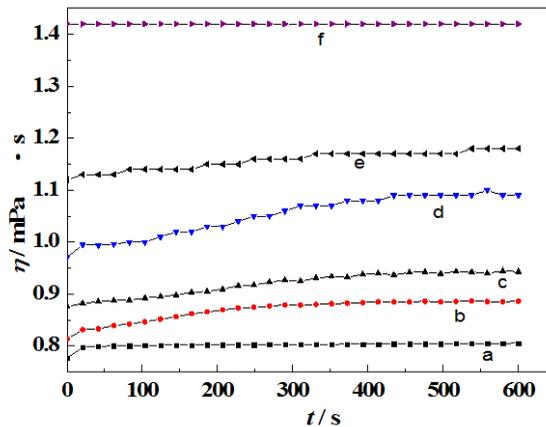
Figure 4: Flow behaviors of crosslink polyacrylamide microspheres dispersed system with different concentration  $\rho(\text{microsphere})/(\text{mg}\cdot\text{L}^{-1})$ : a. 50; b. 100; c. 300; d. 600; e. 900; f. 1500.
