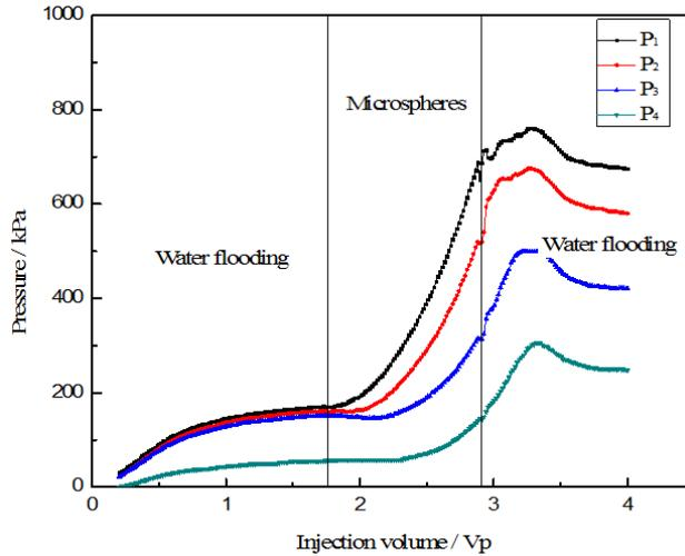
Figure 6: Relationship of pressure and injection volume of crosslink polyacrylamide microspheres dispersed system.
