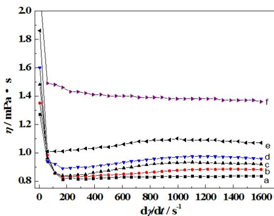
Figure 3: Viscosities of crosslink polyacrylamide microspheres dispersed system with different concentration  $\rho(\text{microsphere})/(\text{mg}\cdot\text{L}^{-1})$ : a. 50; b. 100; c. 300; d. 600; e. 900; f. 1500.
