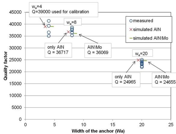
Figure 2: LE resonator: experimental data and results of simulations for different  $w_a$ ; orientation [110],  $L_p = 310\mu m$
