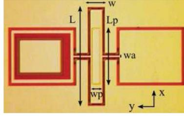
Figure 1: Length extensional resonator Rosenberg, Jaakkola, Dekker, Nurmela, Pensala, Asmala, Riekkinen, Mattila, and Alastalo (2008)
