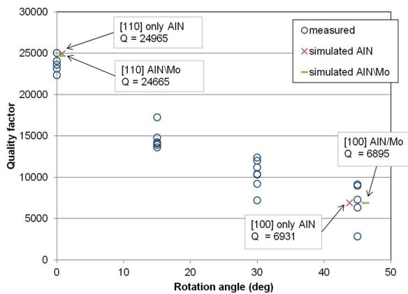
Figure 3: LE resonator: experimental data and results of simulations for different silicon orientations;  $w_a = 6\mu m$ ;  $L_p = 310\mu m$
